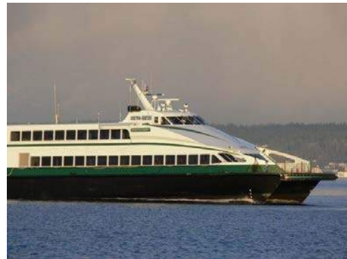
Figure 3 – M/V SNOHOMISH bow extension for auto-slip docking
