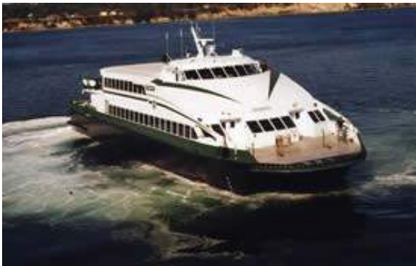
Figure 3 – M/V SNOHOMISH bow extension for auto-slip docking
