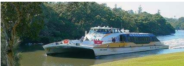
Figure 5 – Australian 230-passenger ferry M/V SHANE GOULD with a wide wet deck and beam
