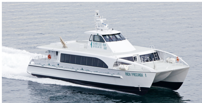
Kitsap Transit's 118-passenger fast ferry is built to minimize wake in Rich Passage.
