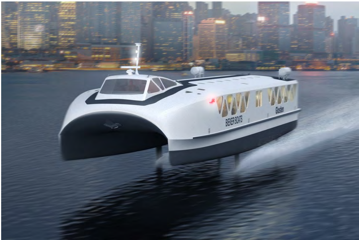
Concept of an all-electric high speed foil vessel under study
